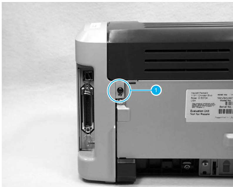
Figure 5-5. Removing the right side cover (2 of 5)
