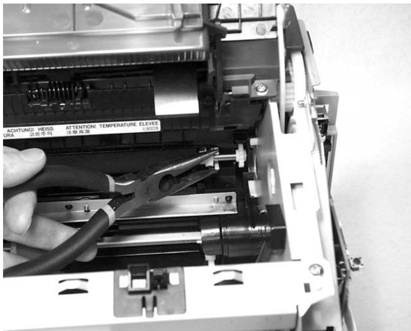
Figure 5-19. Removing the transfer roller (3 of 3)
